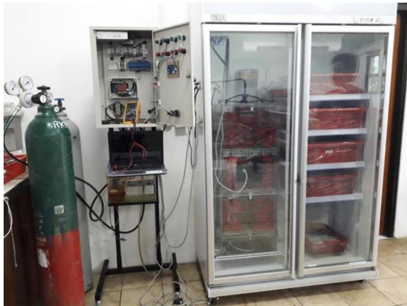
Gambar 17. Mini- controlled atmosphere storage
